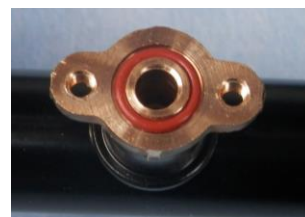
GAS CONTROL VALVE SEAT AND O RING. PHOTOGRAPH 37.
