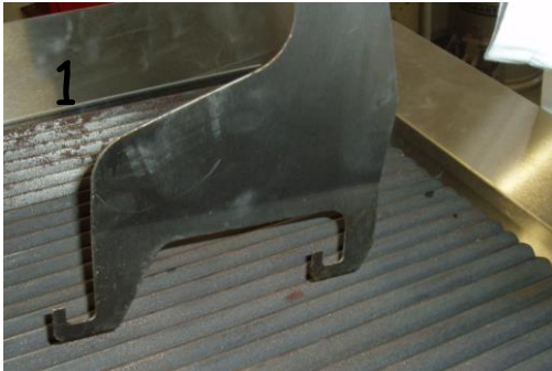
GRATE LIFTING TOOL. PHOTOGRAPH 14.
