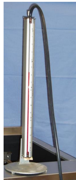
PHOTOGRAPH 22. GAS INLET PRESSURE MANOMETER.
