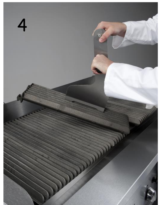
GRATE REMOVED FROM THE CHAR BROILER. PHOTOGRAPH 17.
