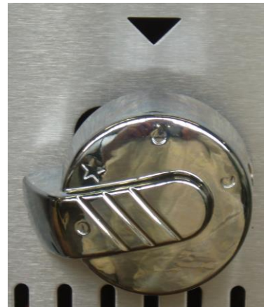
MAIN BURNER 'ON' FULL FLAME POSITION. PHOTOGRAPH 7.
