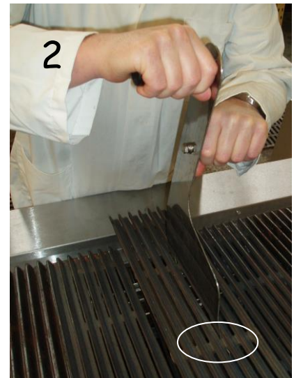
LOCATING THE LIFTING TOOL ON THE GRATE RIBS. PHOTOGRAPH 15.
