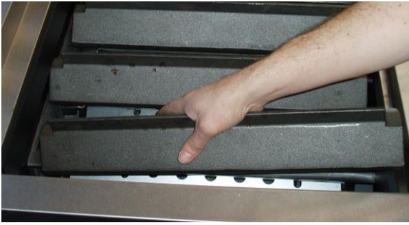
REPLACING THE RADIANTS. PHOTOGRAPH 5.
