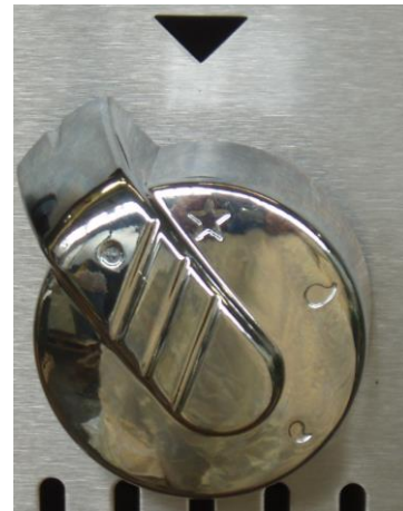
PILOT BURNER 'ON' POSITION. PHOTOGRAPH 3.
