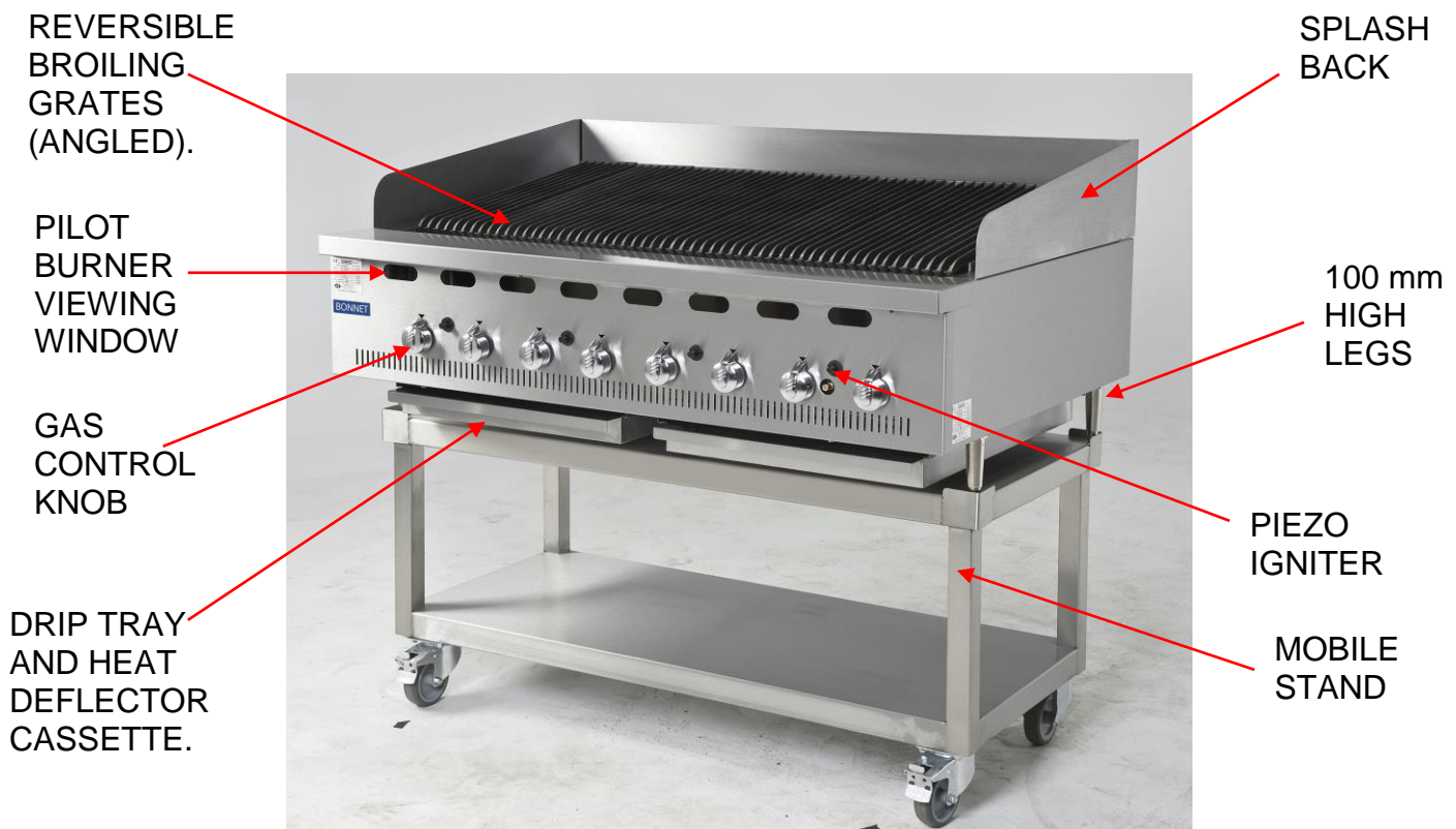
BCB BONNET CHAR BROILER COMPONENT IDENTIFICATION. PHOTOGRAPH 1.
