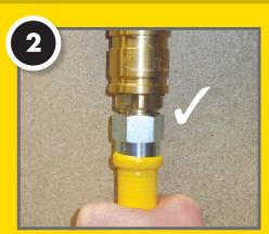
Holding the QD coupling and the hose, push the hose end upwards until the QD collar clicks and engages.
