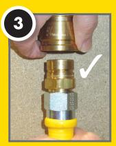
Firstly isolate the gas supply by turning the local isolation valve to the 'closed' position. Grip the outer collar of the QD coupling and, whilst holding the hose, pull back the collar to release the inserted male part.
